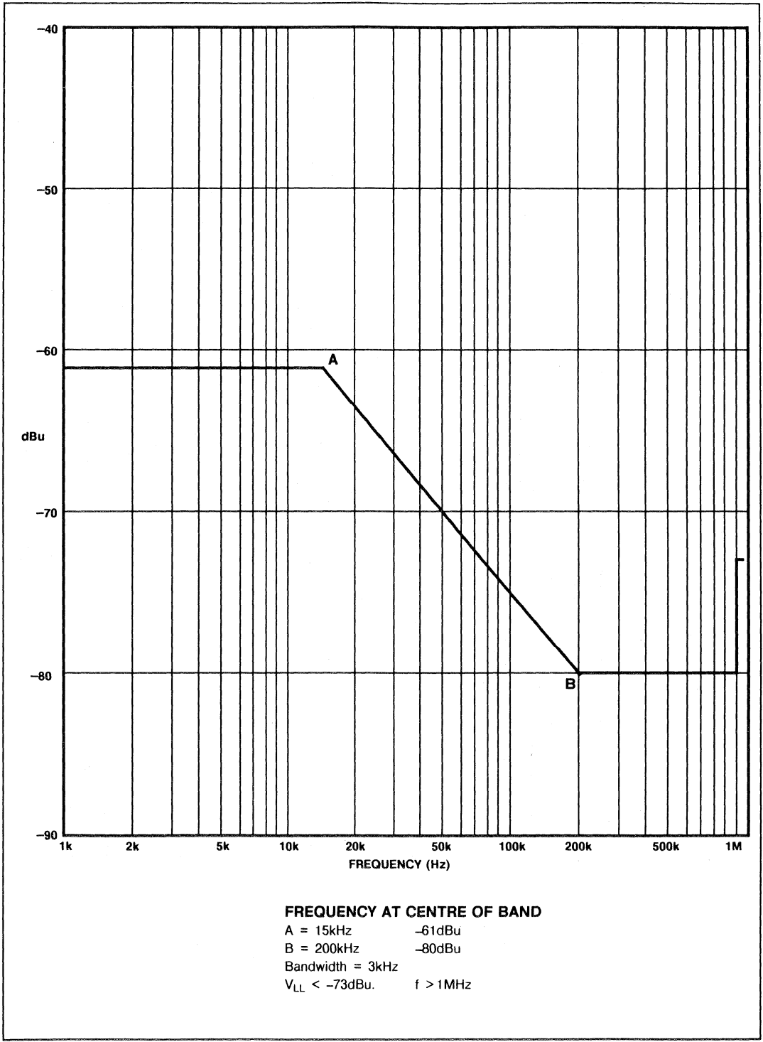
Fig.20 2-Wire longitudinal noise
